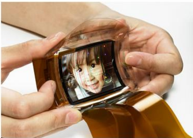
A Flexible OLED Display driven by organic transistors
